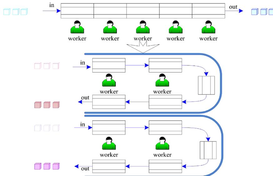
Fig. 1. An example of cell formation in line-cell conversion towards reducing worker(s).
