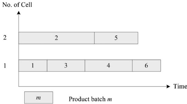
Fig. 2. An example of FCFS scheduling in a cell system (Yu et al., 2012).
